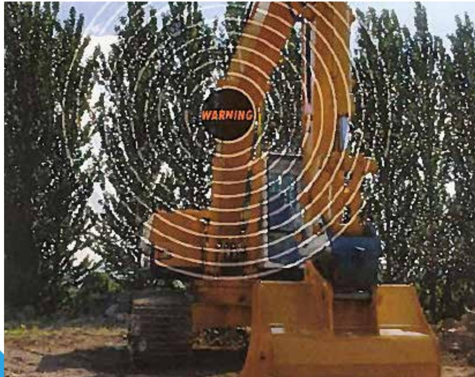
Using the same external sounder as the superior AWS system, the ECS monitors coupler pressure only, alerting individuals in the area that an attachment change is taking place, without the constant monitoring of the excavator and coupler hydraulics.
