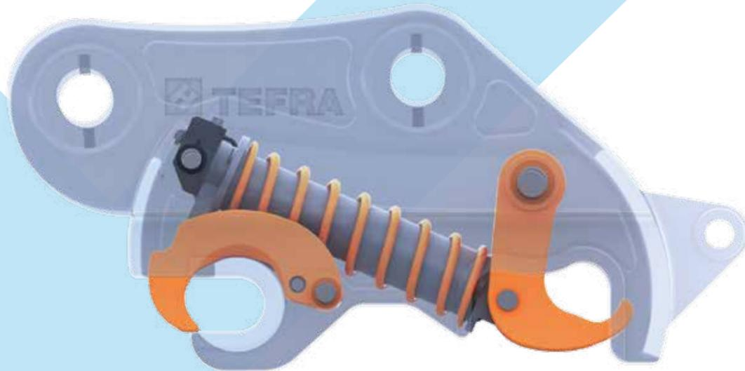
The primary safety system consists of a uniquely designed set of hooks powered by a single high specification hydraulic cylinder. The cylinder works together with a dedicated solenoid valve, locking the attachment securely into place.
