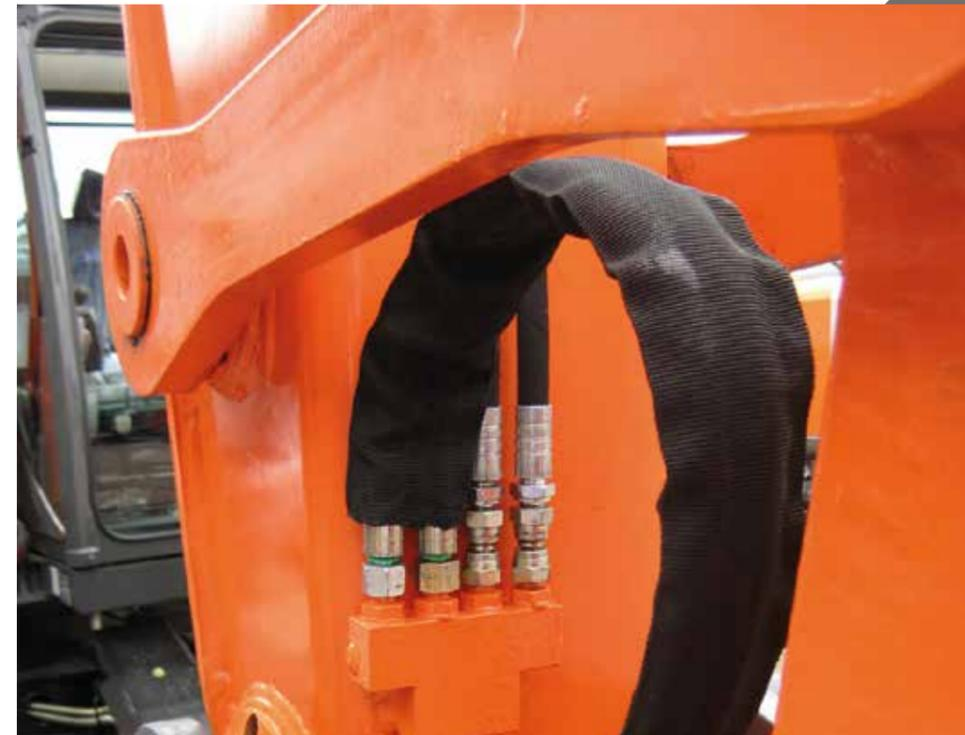
It's long been an issue that coupler hoses are vulnerable due to their location. They can easily become entangled in the excavator linkage, causing rapid wear and tear, often causing major damage to the hoses.
