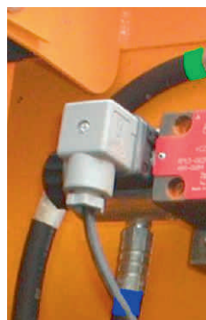
Wired DIN connector showing YELLOW/BLACK multicore cable from switch box in cab
