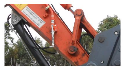
Hoses should be suitable routed from the ram ports to the double acting circuit. Normally this will be the quick release fittings on the hammer circuit however an independent circuit may also be used. Care should be taken so that the hoses cannot become entangled in the thumb or other attachments and should be routed such that the will not rub or chafe on any moving parts.
